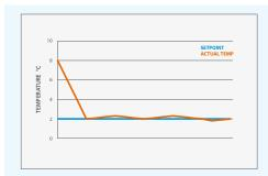
Daikin Inverter driven systems are designed to maintain a constant cabinet temperature, rather the fluctuating temperatures found in standard systems [shown above].
